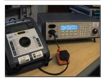
Residual circuit breaker testers manufactured by many companies are designed to test and measure the break time of AC mains (RCB) trips at set test currents. To do this they allow a fault current to pass between live phase and earth. The 'fault' current is started by pressing a button on the tester, usually an LCD counter on the tester measures the time in milliseconds until the mains supply is disconnected.
