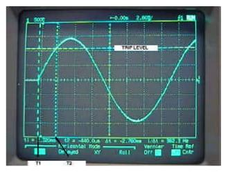
The diagram above shows the start of the fault current from an RCB tester. The test button would have been pressed at a point in the previous cycle PRECEDING the point T1 - up until then there would either have been no current or with some testers a PRE-TEST current below the trip current level.
